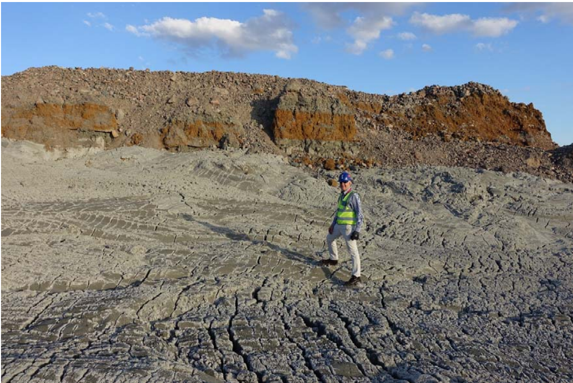
Photo B8-9: Eastern side of slump showing basal clay layer to Stage 4 or above.
