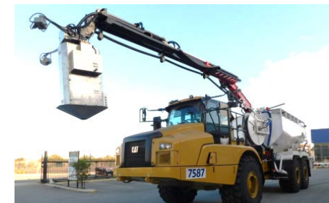
Robotic explosive placement
